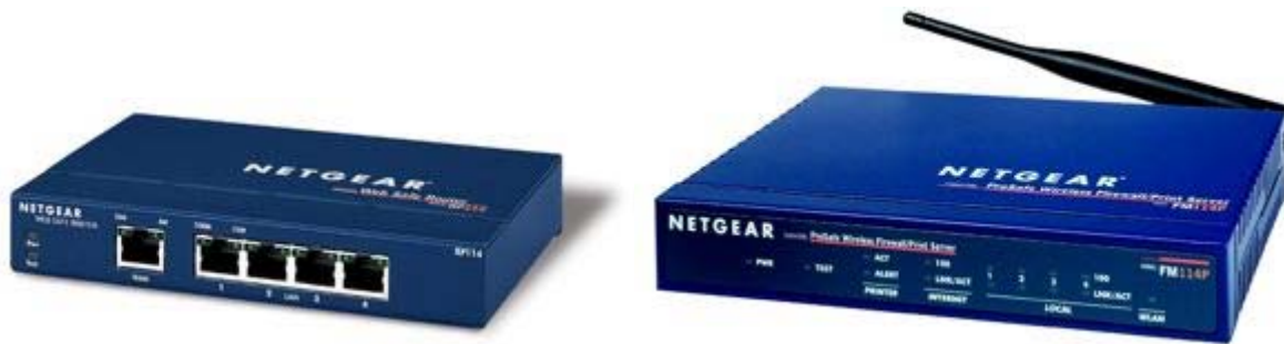
Abbildung 6: links LAN Router, rechts WLAN Router
